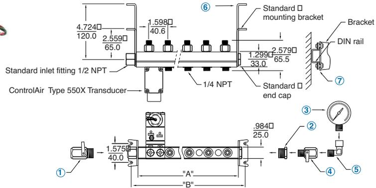
The Type 925 Multifunction Manifold provides a common air supply line to multiple units of our Type 550X and Type 900X I/P, E/P transducers.
