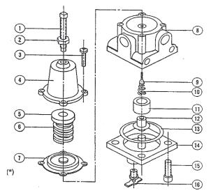
All items marked with an asterisk (\*) will be included in the repair kit. Other parts may be ordered separately by specifying the item number, part name, and the part number of the regulator for which the parts are intended.
