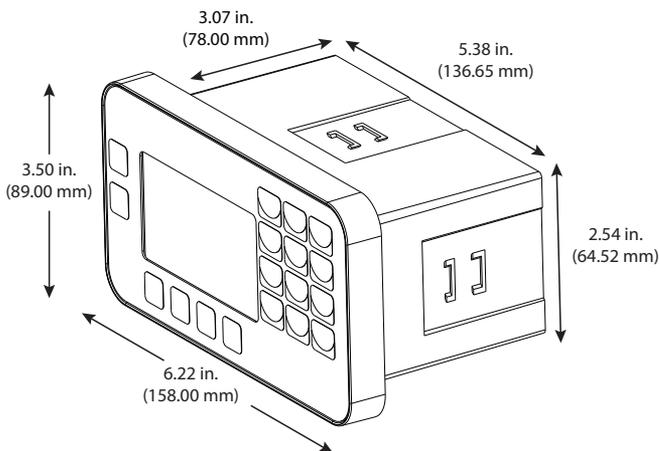
Figure 2: Mounting dimensions
