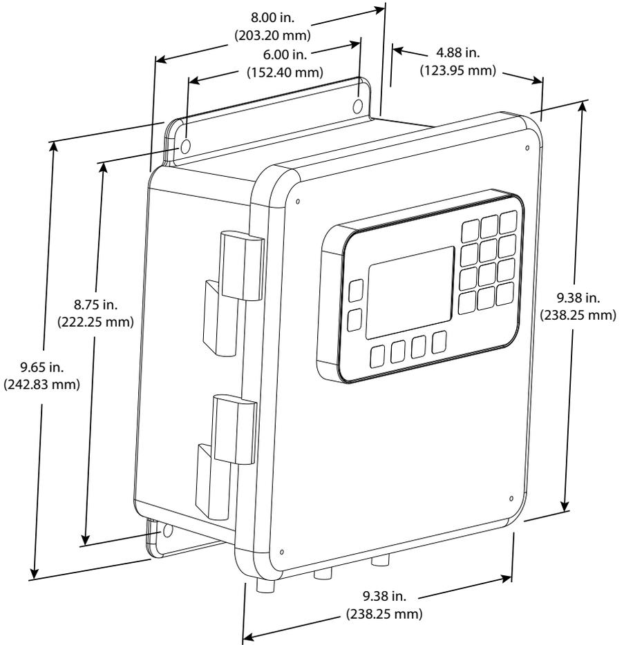
Figure 3: FC-5000 BTU Monitor in an enclosure
