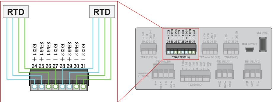
**NOTE:** The wires in your application may not be the same color as the wires in the diagram. The number of each color represents the number of a color of wire that your application will have. For example, the 3-Wire RTD diagram has two green wires and one blue wire. Your application may have two yellow wires and one red wire. To wire the system you would wire the two yellow wires the same way the green wires are in the diagram, and the same with the red and blue wires.
