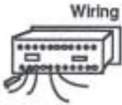
The rear panel of the CB 20 controller contains 15 active screw terminals for connecting #28 to #14 guage insulated stranded wire (#18 guage stranded wire is recommended).
